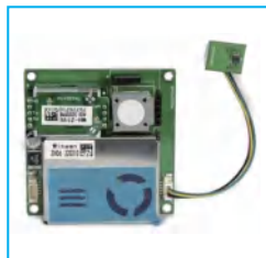
Air Quality Sensor (Co2/Humidity/VOC)
